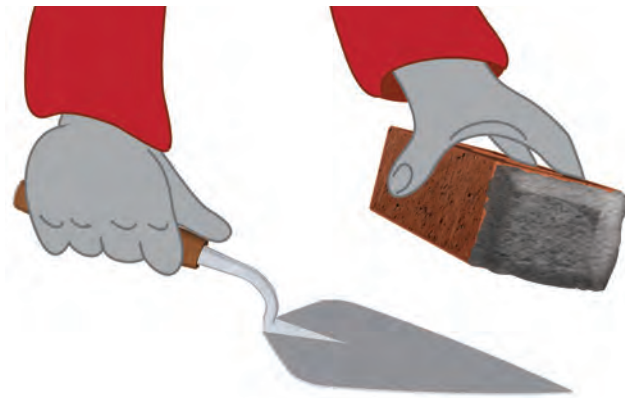
11.7 - Lifting enough mortar to butter a brick.
