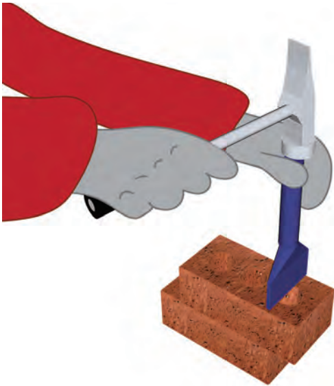
11.4 - When cutting face-bricks greater accuracy is generally required than with the stock bricks (as the latter is normally plastered over). A bolster is used to ensure that the brick breaks at the desired point.
