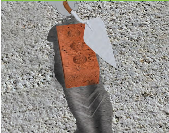
11.6 - Showing mortar bed slightly furrowed to make the placing of the brick easier to lay.
