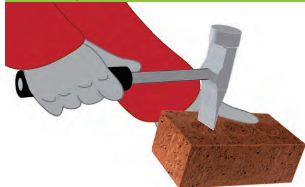
11.2 - Cutting a half brick with a brick-hammer.
