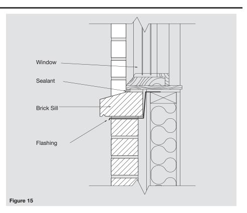
be so saturated with water that the water appears inside of the structure. Four inches of brick masonry, the usual nominal thickness of a brick veneer, will not keep the water out all of the time; the mass of masonry is not so great that it can absorb all of the water to which it is exposed before penetration through the brick wythe occurs.
