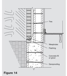
external flashing. Masonry copings tend to be more susceptible to water penetration, require through-wall flashing, and may require more maintenance because of reliance upon sealants in movement joints between adjacent members. Note that covering the exposed face of the backup with an impervious membrane for the entire height of the back-up wythe may trap moisture within the back-up wythe and
