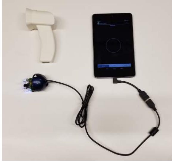
Figure 7-1: The imaging device consists of a webcam with six infrared LEDs, as well as a hood attachment that covers the webcam. The device is connected to a mobile device which is running the companion mobile application.
