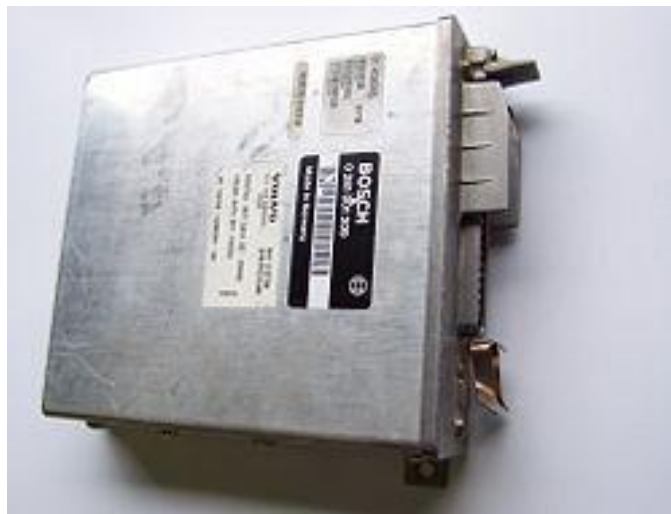
EDC control unit
