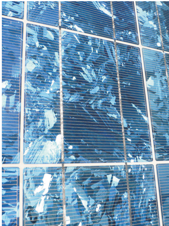
Fig. 10. Polycrystalline PV cells laminated to backing materials in a PV module. Credit, Georg Slickers. http://upload.wikimedia.org/wikipedia/commons/1/15/Polycrystalline-silicon-wafer_20060626_568.jpg
