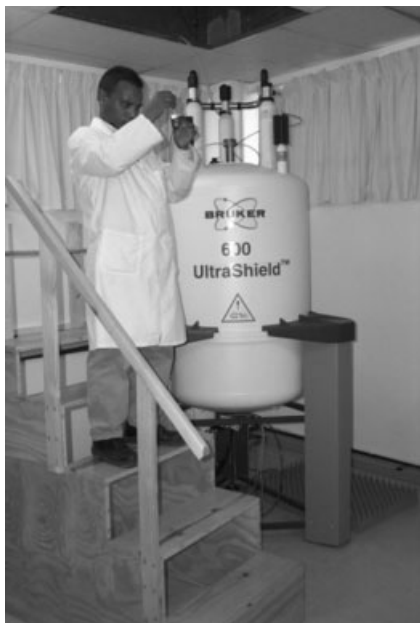
Figure 1.11 600 MHz NMR forming part of the NABSA analytical service at the University of Gabarone, Botswana. Photo from B.M. Abegaz.
