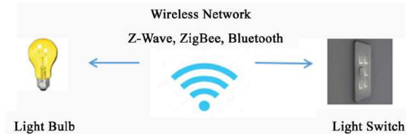
Figure 15. Example of device-to-device communication model.
