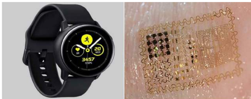
Figure 12. Smart watches and fitness trackers in left, Embedded skin patch in right.
