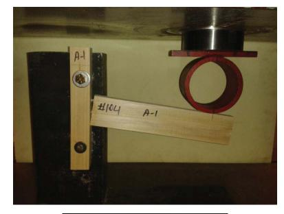
Failure on the T-shaped screw joints
