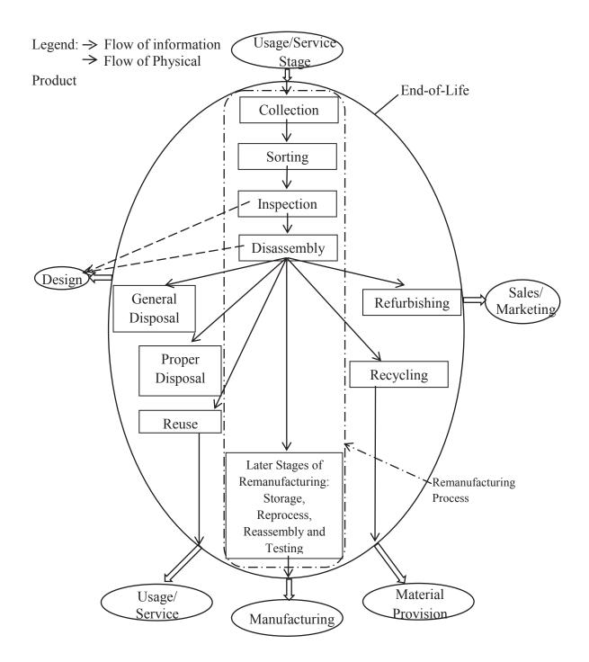
Figure 2-4: Decomposition of product EOL Stage (Lee et al., 2001).
