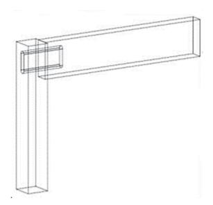
Figure 3-19: Glued rectangle mortise and tenon L-joint configuration.
