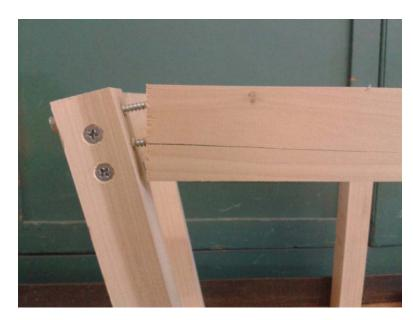
Failure on the stools with bed bolts (with dowel nuts) joints.
