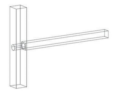
Figure 3-18: Glued round mortise and tenon T-joint configuration.
