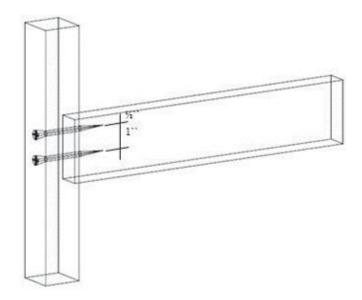
Figure 3-13: Screw T-joint configuration.
