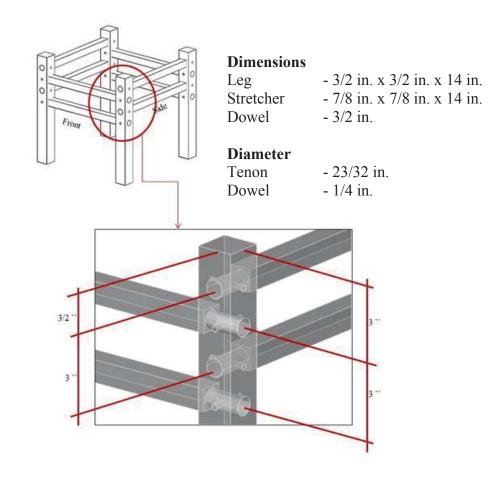
Figure 3-7: Pinned round mortise and tenon joint, two stretcher frame construction.
