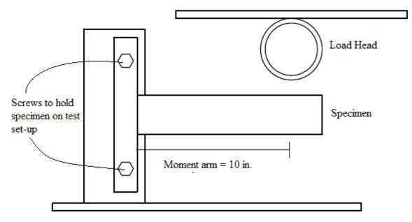
Figure 3-21: Static load test set up.
