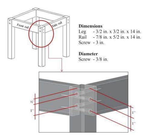
Figure 3-5: Screw joint frame construction configuration.
