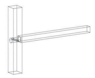
Figure 3-15: Pinned round mortise and tenon T-joint configuration.
