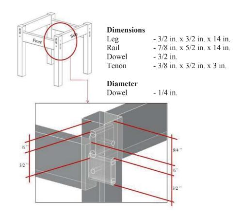
Figure 3-9: Pinned round-shouldered rectangular mortise and tenon joint frame construction configuration.
