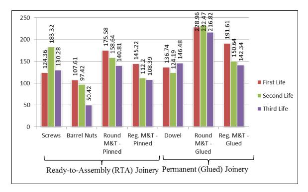
Figure 3-23: Average load caring capacity of the stools with different joinery systems in each life.
