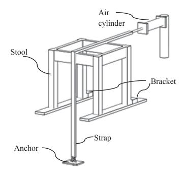
Figure 3-22: Cyclic front-to-back load test configuration.
