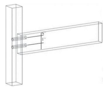
Figure 3-17: Dowel T-joint configuration.
