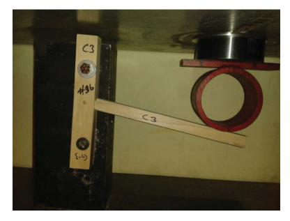
Failure on the T-shaped pinned round mortise and tenon joints
