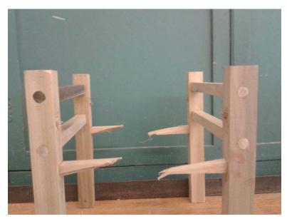
Failure on the stools with glued round mortise and tenon joints.
