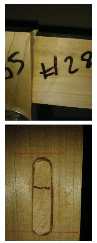
Failure on the L-shaped glued rectangular mortise and tenon joints
