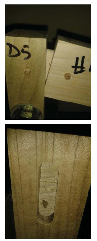
Failure on the L-shaped pinned rectangular mortise and tenon joints
