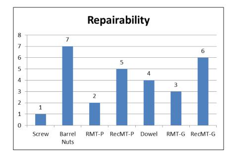
Figure 3-25: Reparability level of stool (easiest – 1 to hardest – 7)
