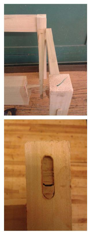
Failure on the stools with glued rectangular mortise and tenon joints.
