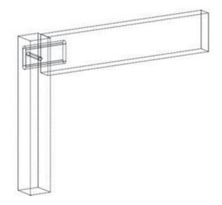
Figure 3-16: Pinned rectangle mortise and tenon L-joint configuration.
