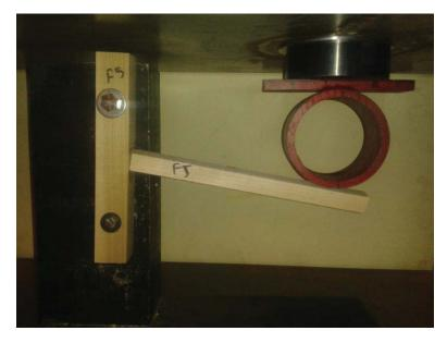
Failure on the T-shaped glued round mortise and tenon joints
