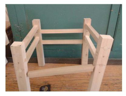
Failure on the stools with pinned round mortise and tenon joints.
