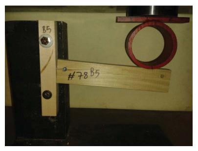
Failure on the T-shaped bed bolts (with dowel nuts) joints
