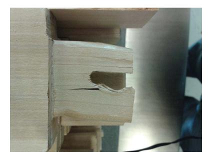
Failure on the stools with dowel joints.
