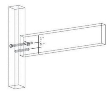
Figure 3-14: Bed bolts (Dowel nuts) T-joint configuration.
