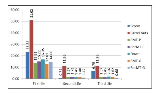
Figure 3-24: Material cost of stools in each life (In the second life and the third life, only new material cost – U.S. Dollars (\$))
