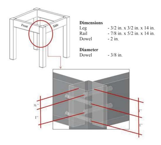
Figure 3-11: Dowel joint frame construction configuration
