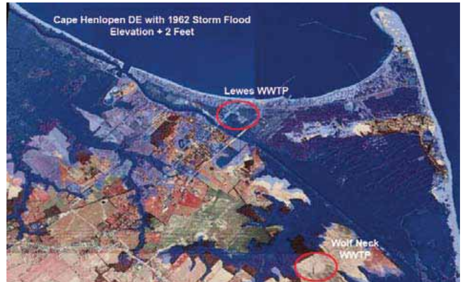
Fig. 1.23. Wastewater treatment plants in the area of Cape Henlopen DE are vulnerable to sea level rise. Using the 1962 storm flood elevation, this image shows that Lewes WWTP would be flooded and the facility at Wolf Neck would be nearly surrounded by water. Courtesy of David B. Carter, Coastal States Organization Climate Change Workgroup Co-Chair & Delaware Coastal Program Manager.
