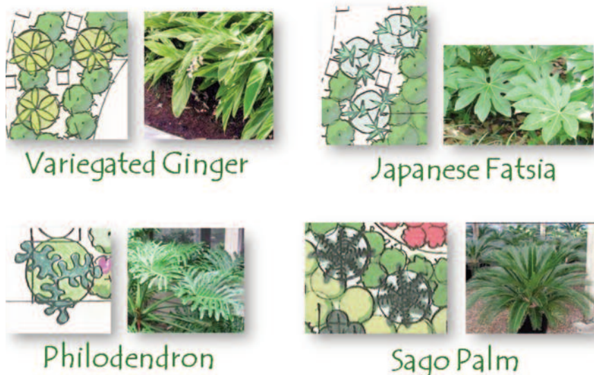
Figure 30. Plan symbols may be modified to reflect texture or other plant characteristics. This allows the species to be quickly recognizable when you are reviewing your planting plan. Image and planting symbols by Pat Drackett.
