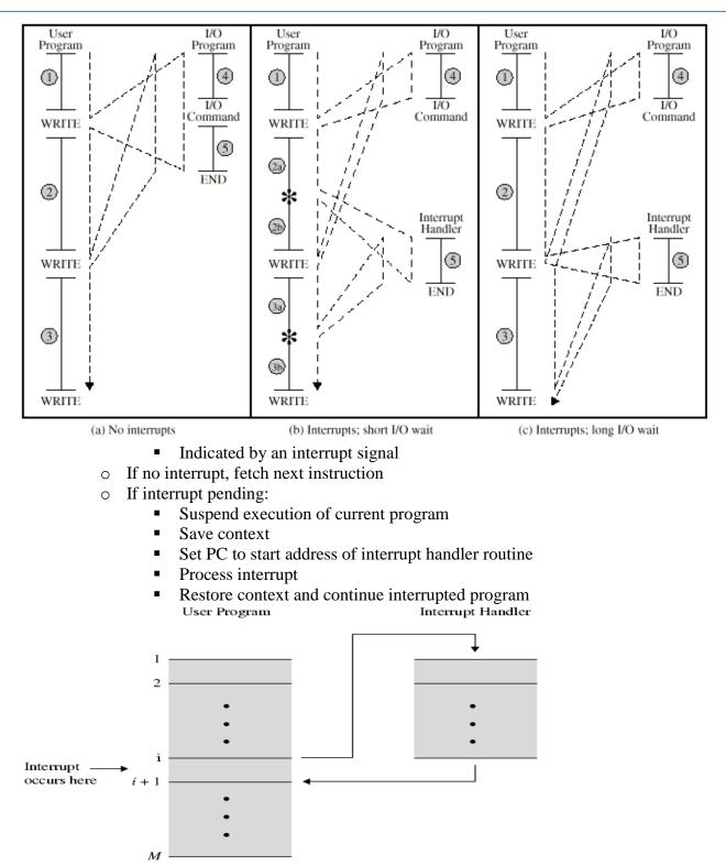
Fig: Transfer of control via interrupts
