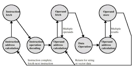
Fig: Instruction cycle state diagram
