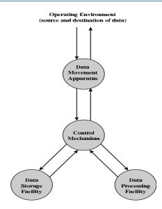
Fig: Functional view of a computer
