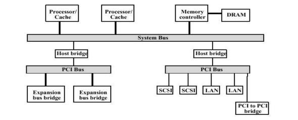
Note: In a multiprocessor system, one or more PCI configurations may be connected by bridges to the processor's system bus.
