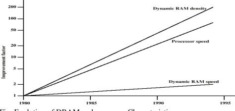
Fig: Evolution of DRAM and processor Characteristics
