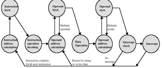
Fig: Instruction cycle state diagram, with interrupts
