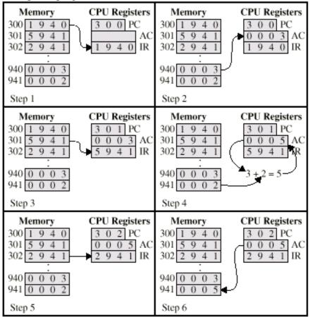
Fig: Example of program execution (consists of memory and registers in hexadecimal)
