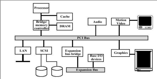
Note: Bridge acts as a data buffer so that the speed of the PCI bus may differ from that of the processor's I/O capability.
