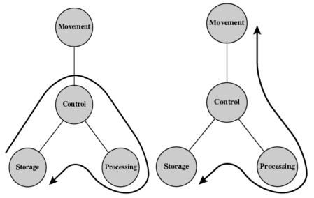
Fig: Processing from / to storage Fig: Processing from storage to i/o
