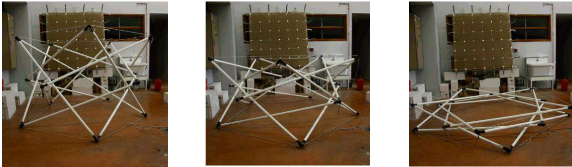
Figure 8.3.5: Folding a tensegrity ring ©N.A. Dung
