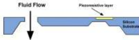
Figure 36. Micromachined mechanical (drag-force) flow sensor [39].
