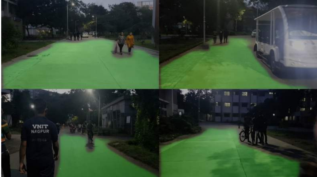
Figure 6.8: Results of ENet trained with Cityscapes dataset on VNIT campus images with green overlay representing the detected road pixels.
