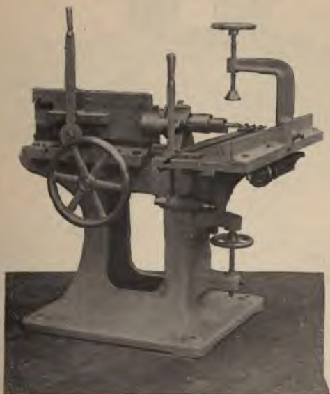
FIG. 259.—Chain Cutter Mortising Machine.
