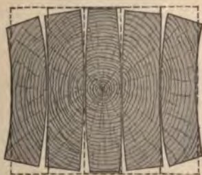
FIG. 8.—Effect of shrinkage of a balk sawn into planks.
