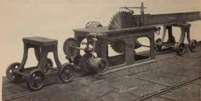
FIG. 241.—Circular Saw Bench with Rope Feed.
