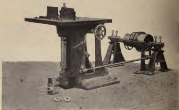
FIG. 253.—Vertical Spindle Circular Moulding Machine.
