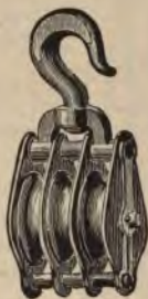
FIG. 635.—Three-Sheaved Pulley Block.
