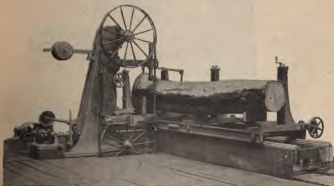
FIG. 234.—Heavy Band Saw for cutting Logs and Balks.
