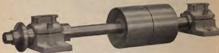
FIG. 238.—Circular Saw Shaft and Bearings.
