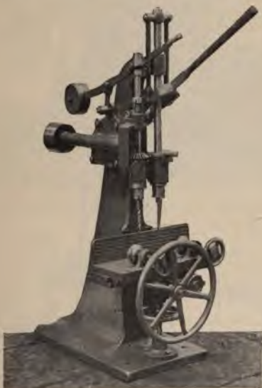
FIG. 257.—Mortising and Boring Machine.
