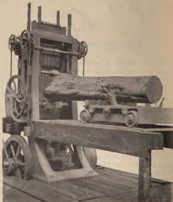
FIG. 227.—Vertical Log Frame Saw.
