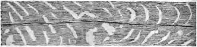
FIG. 1.—Sketch showing the appearance of silver grain in a radial longitudinal section of Oak.
