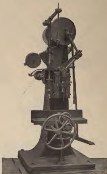
FIG. 258.—Power Mortising Machine.
