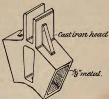
FIG. 454.—Sketch of Cast-iron Connection at Upper Ends of Principal Rafters and King-rod.
