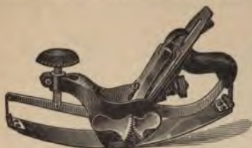
FIG. 196.—Adjustable Compass Plane.
