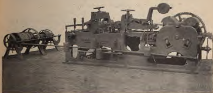
FIG. 252.—Planing and Moulding Machine.
