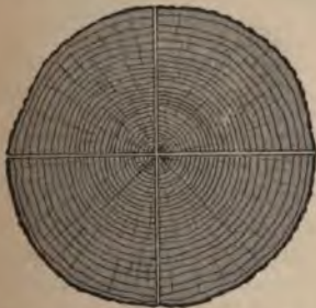
FIG. 5.—Method of quartering a log.
