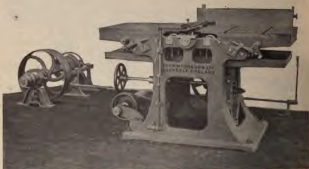
FIG. 250.—Surface Planer and Thicknessing Machine.
