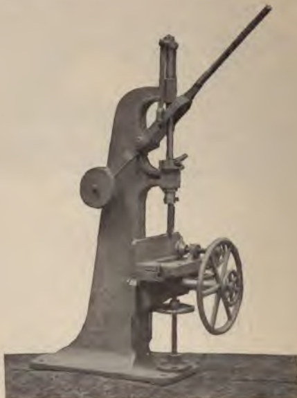
FIG. 256.—Lever Mortising Machine.
