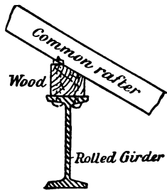
FIG. 420.—Iron Girder supporting Common Rafter.
