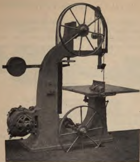
FIG. 236.—Band Saw with Motor.
