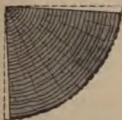
FIG. 9.—Effect of shrinkage upon a quarter of a log.
