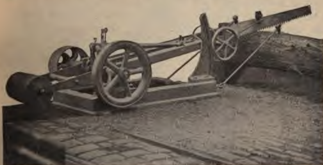
FIG. 233.—Reciprocating Cross-cut Saw.
