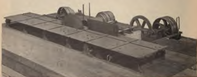
FIG. 242.—Circular Saw Bench with Movable Table.
