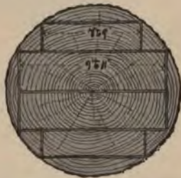
FIG. 6.—Method of converting a soft-wood log.
