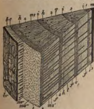
FIG. 4.—Portion of a four-year-old stem of the Pine, cut in winter. 1, 2, 3, 4, the successive annual rings of the wood; b , bast; br , bark; c , cambium; s , spring wood; h , resin canals; i , junction of wood of successive years; m , pith; ms , medullary rays; a , autumn wood. (Four times natural size.)
