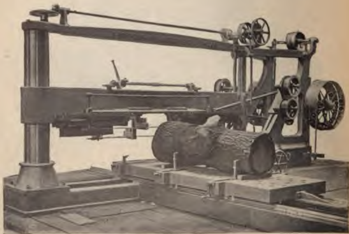
FIG. 232.—Horizontal Log Frame Saw.
