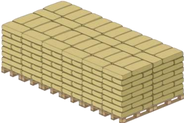
Figure 2: Bonded or interlaced stack
