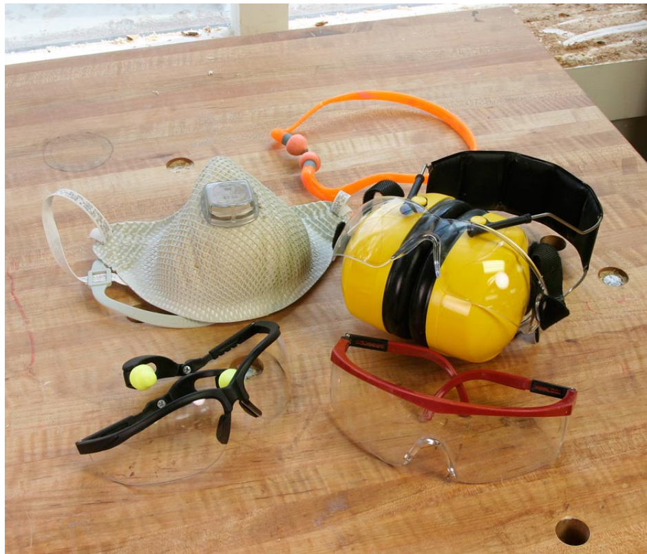
Safety gear – safety glasses, hearing protection and some type of dust mask – should always be used when routing.
