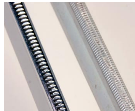
The teeth on the left are on the cheaper clamp. They're coarser and are only on a small portion of the bar. The teeth on the right are finer and there's more of them.
