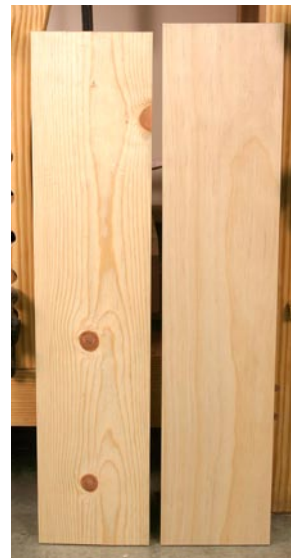
This clearly shows the difference between the #2 pine and the prime grading of the same species.
