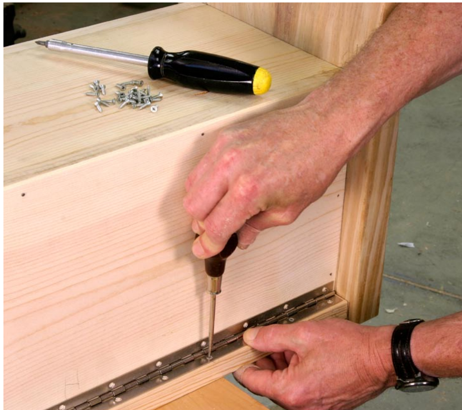
When installing a piano hinge, first install just a few of the screws. Then test the hinge.
