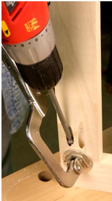
The long driver bit that comes in the kit keeps the drill chuck away from the wood.
