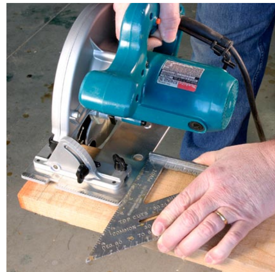
Aligning the blade with the cut line and using a speed square provides a temporary fence for a square or straight cut.
