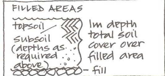
DIAGRAM SHOWING FORMATION LEVELS PLUS MINIMUM DEPTHS OF TOPSOIL FOR DIFFERENT TYPES OF PLANTING
