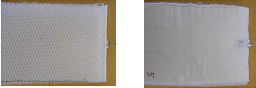
Figure 5. A three layer construction of samples 5a and 5b.
