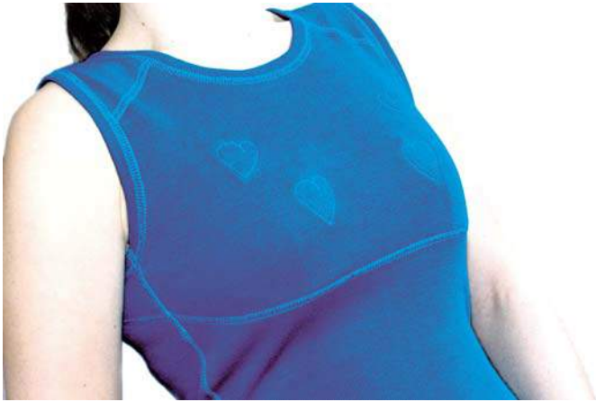
Fig. 1 Example of a prototype T-shirt housing smart textile based ECG-electrodes. Commercially available dry electrodes were housed in a padded structure over the shoulder, i.e. over the trapezius muscle.
