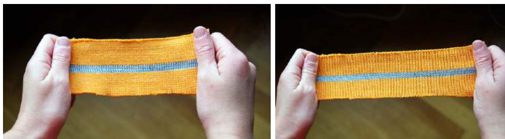
Figure 32. Conductive elements approaching each other respectively separating from each other
