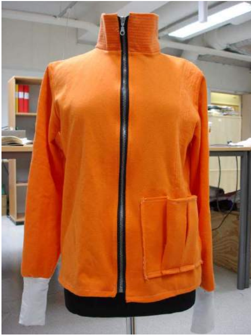
Fig. 6 Prototype for ECG monitoring in home health care situations. ECG signals are registered using textile electrodes integrated in the left and right wristlet.
