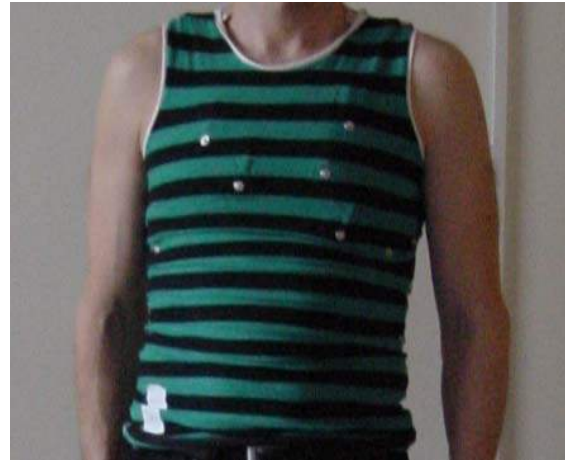
Figure 1. The prototype T-shirt housing smart textile based ECG-electrodes
