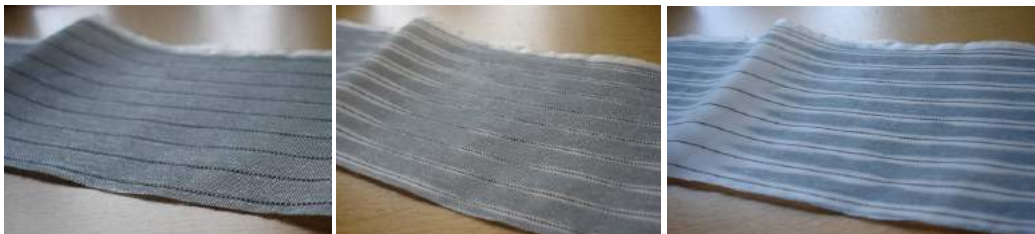
Figure 37. Thermochromic print on a woven heating fabric
