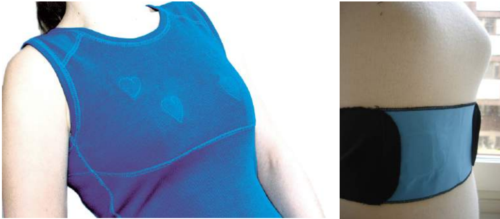
Figure 58. Shirt and belt for heart rate monitoring
