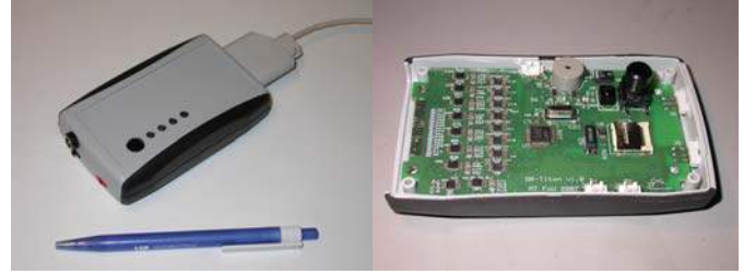
Fig. 2 Left photo: 8-channel Bluetooth acquisition prototype unit. Right photo: The modular-constructed acquisition unit containing, CPU, signal conditioner (incl. A/D converters), bluetooth (for real-time transmission) and memory-card (for possible logger functionality).
