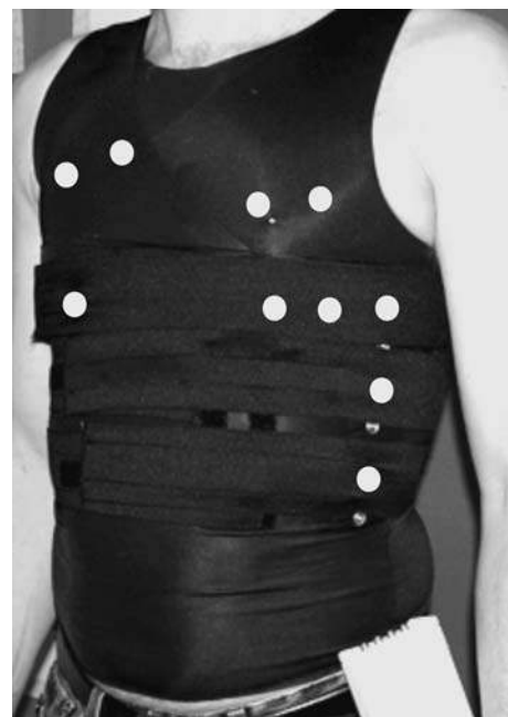
Fig. 1 T-shirt with integrated textile electrodes and the ECG monitor with a wireless transfer of data to a PC. White dots indicate positions of electrodes
