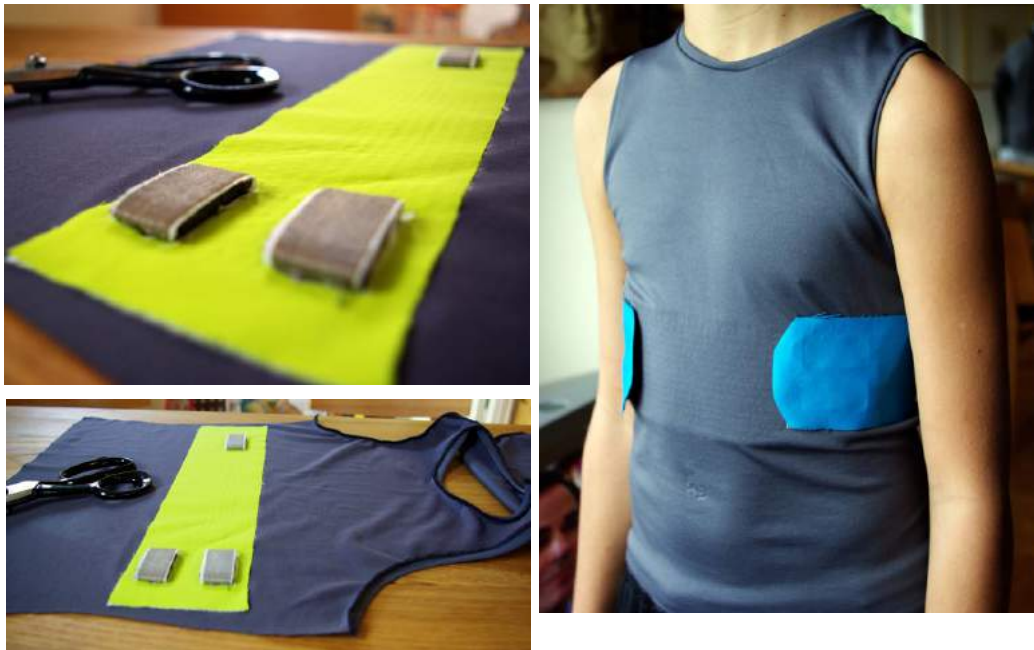
Figure 54. General health monitoring system integrated in a garment
