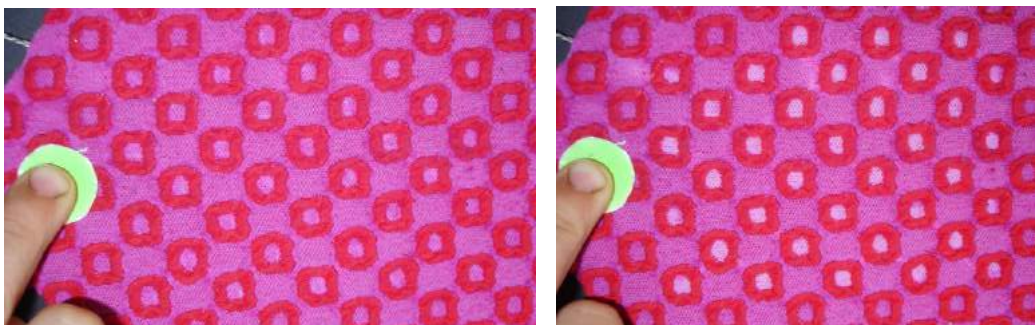
Figure 38 Thermochromic print on a three-layer knit.
