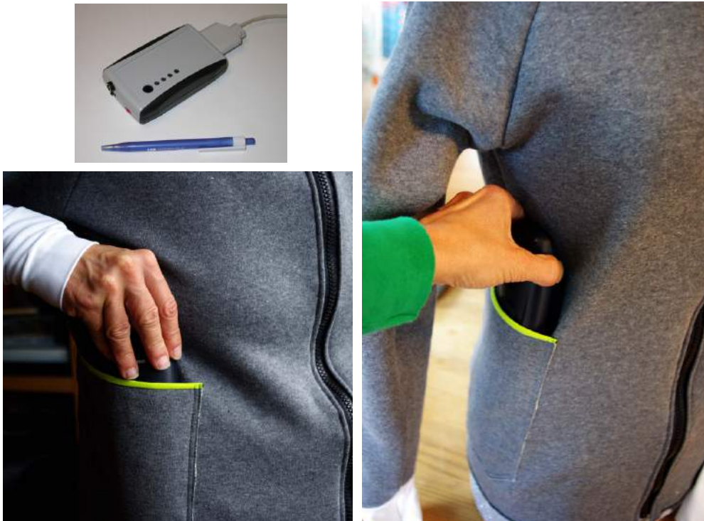
Figure 60. The acquisition unit and its placement in the cardigan
