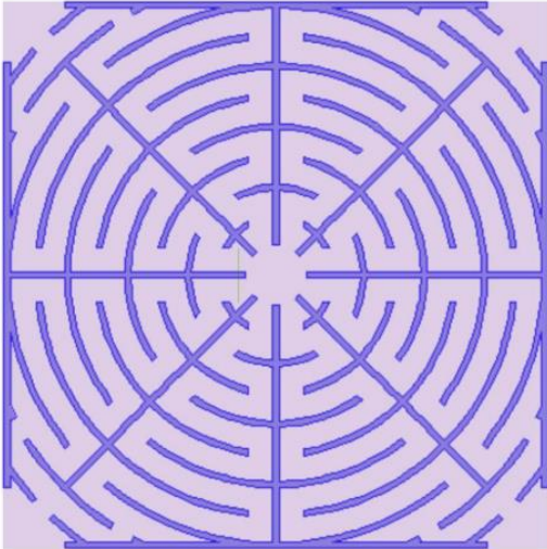
Figure 5: Diagram of spider web-structured labyrinthine acoustic metamaterial.
