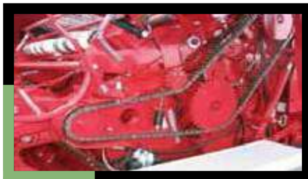
Interlocked guards stop the machine when opened
