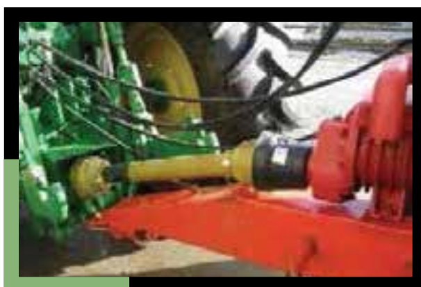
A proper PTO Guard can reduce entanglement risk to Zero
