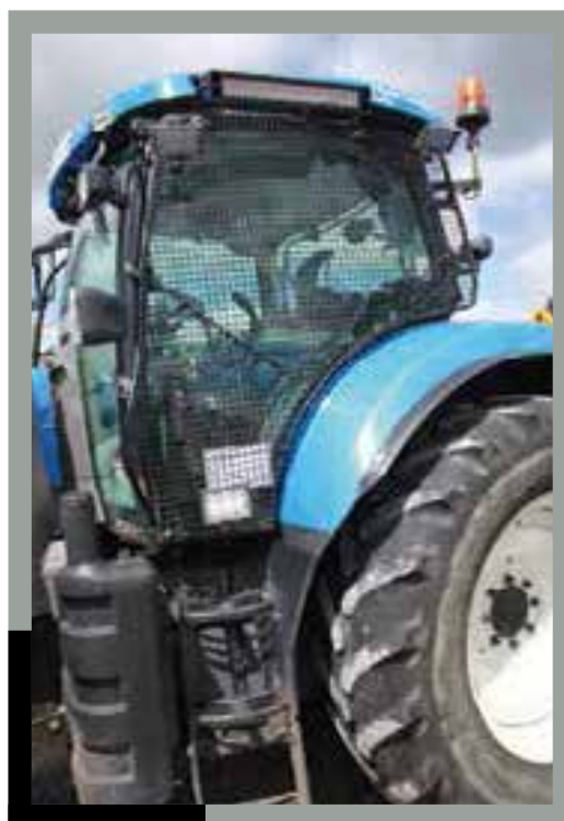
Install mesh on windows to protect from debris
