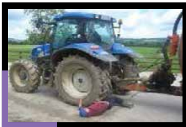
Impact & crushing while reversing is a common cause of fatalities
