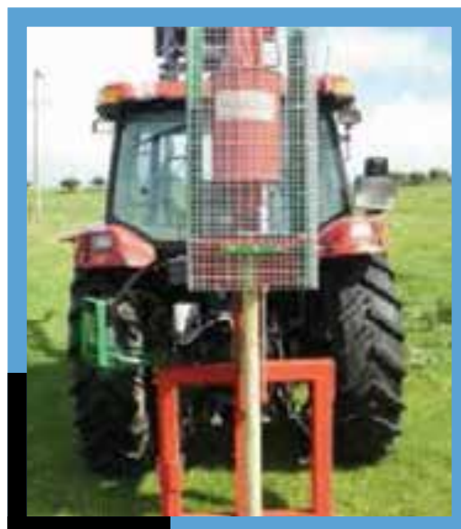
Check that there is adequate guarding on the post driver
