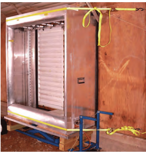
Figure 10. Fan assessment numeration system (FANS) developed by Gates et al. (2005) to describe the performance curve of a ventilation fan in an animal house. The unit can be used on either the inlet or exhaust side of the ventilation fan.
