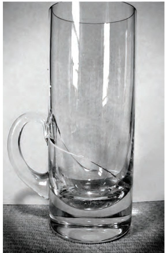
Figure 10. Example of fractured glass (© Scott A. Morris).
