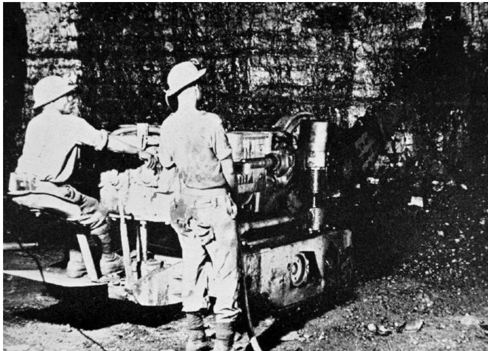
Figure 8. A universal coal cutter being used to prepare large scale coal specimens.
