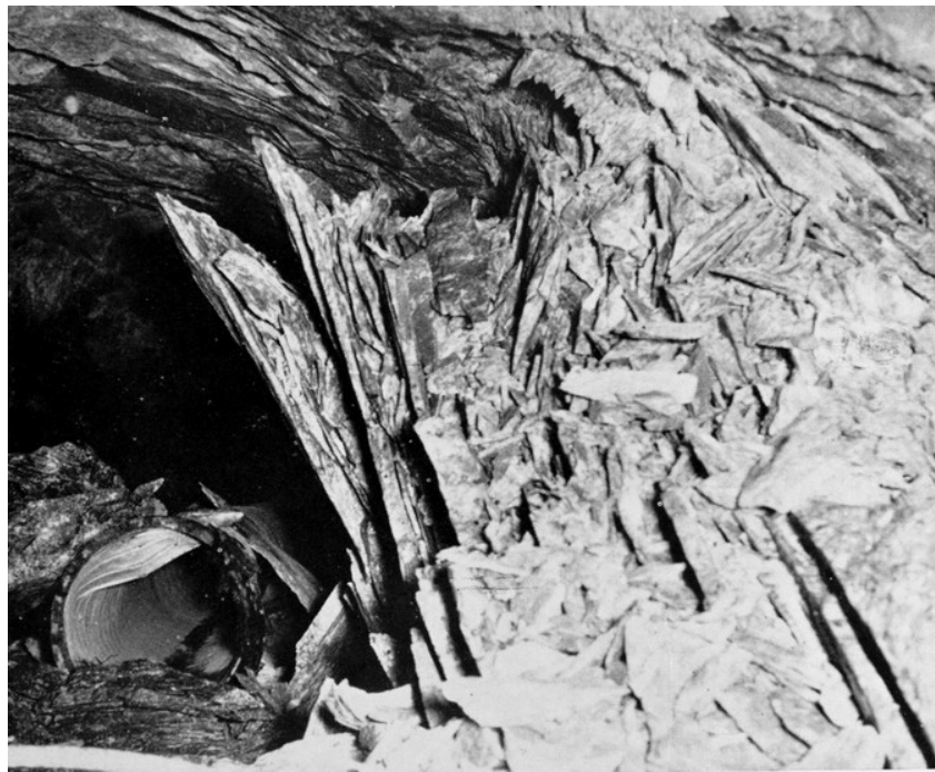
Figure 1. Effects of a rockburst in a deep-level South African gold mine.
