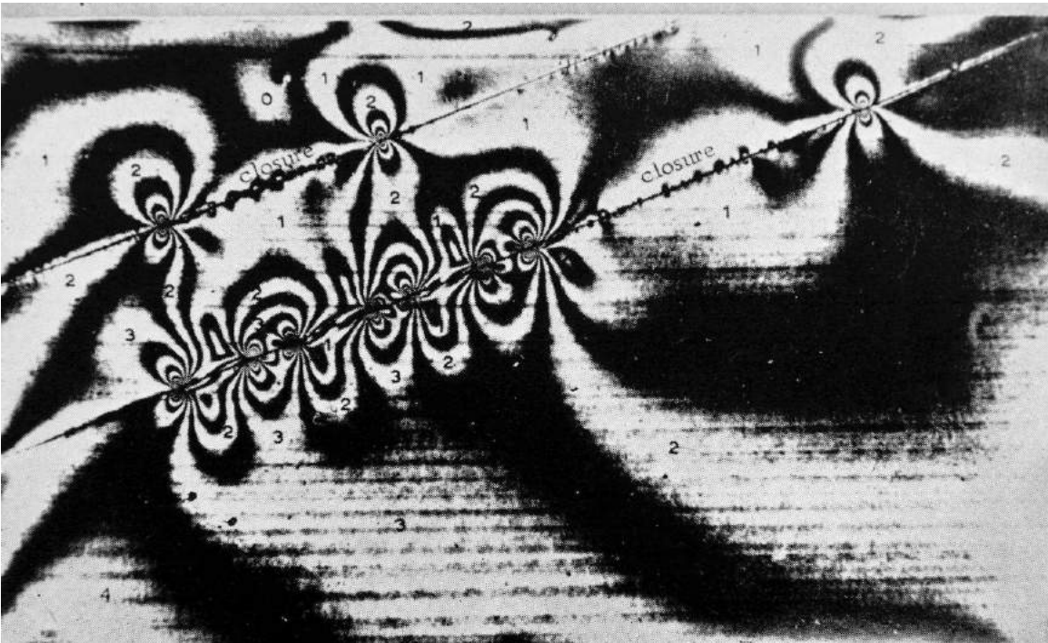
Figure 6. Photoelastic pattern in a min model which was stress-frozen at a centrifugal acceleration of 100 times the acceleration due to gravity.
