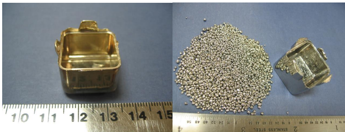
Figure 5. Gold BMG (left) and 850 platinum BMG (right) boxes , both formed by thermoplastic process; also some BMG bead feedstock (from reference 64)
