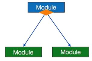
Jump - An arrow is shown pointing inside the module to depict that the control will jump in the middle of the submodule.
