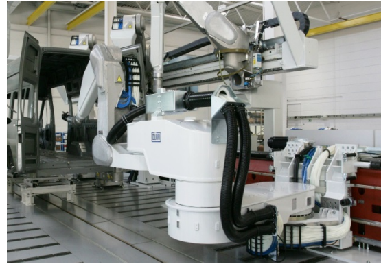
The Swingarm is an articulated robot combined with SCARA elements
