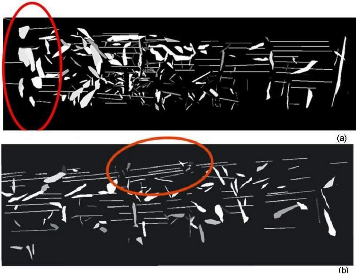
Fig. 19. 2D image of the fractures and drillhole model of the TASQ Tunnel. (a) Left side of the TASQ Tunnel (the floor is in the lower part and the tunnel face is on the right). (b) Right side of the TASQ tunnel (the floor is in the upper part and the tunnel face is on the right).
