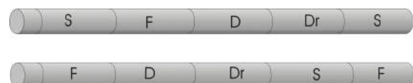
Fig. 11. Example of cyclic sampling of the cores where the (S) is the specimens subject to saline environment, (F) formation water, (D) distilled water and (Dr) are dry conditions.
