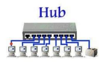
3. Switch: A switch is a network device which is used to interconnect computers or devices on a network. It filters and forwards data packets across a network. The main difference between hub and switch is that hub replicates what it receives on one port onto all the other ports while switch keeps a record of the MAC addresses of the devices attached to it and forwards data packets onto the ports for which it is addressed across a network, that's why switch is intelligent Hub.
