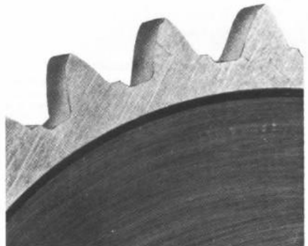
Excessive Wear: Material has been uniformly worn away from the tooth surface causing a deep step. The tooth thickness has been decreased and the involute profile destroyed. Some slow-speed gears can operate on such a profile until so much material has been worn away that the tooth fails under beam bending fatigue.
