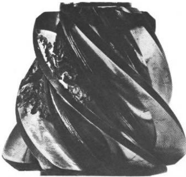
Spalling: This hardened pinion shows an advanced stage of tooth spalling. Material has progressively fatigued away from the surface until a large irregular patch has been removed.
