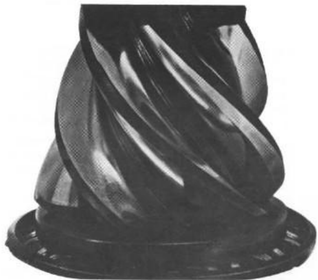
Polishing: Run-in under operating conditions, this hardened hypoid pinion has developed a highly polished surface. Undoubtedly the extreme-pressure additives in the lubricant had a tendency to promote polishing on the tooth surfaces.
