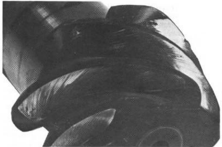
Ridging: On this hardened pinion, note that some wear has taken place and that some surface pitting is present although the predominant mode of failure is ridging.
