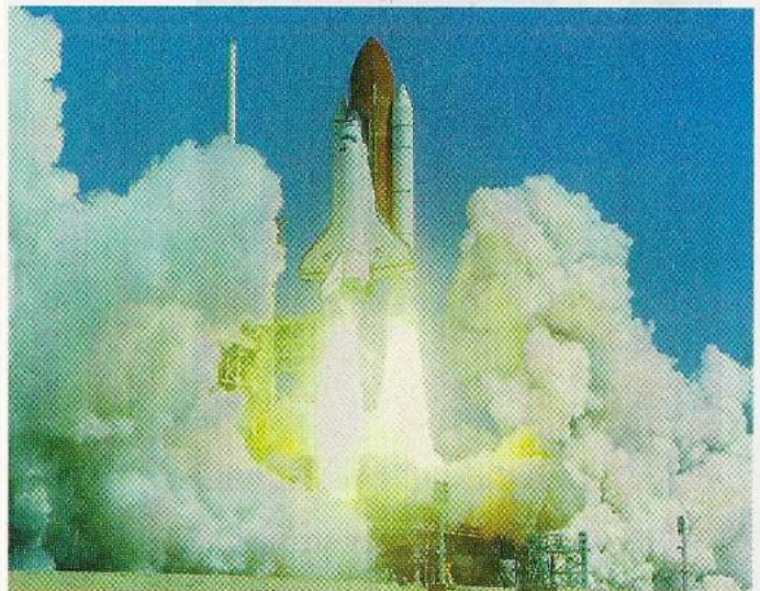
FIGURE 4–10 Another example of Newton’s third law: the launch of a rocket. The rocket engine pushes the gases downward, and the gases exert an equal and opposite force upward on the rocket, accelerating it upward. (A rocket does not accelerate as a result of its propelling gases pushing against the ground.)
