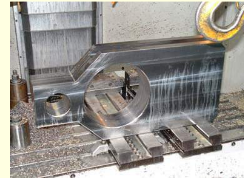
Contournage, surfacage, alésage, rainurage, perçage, taraudage
