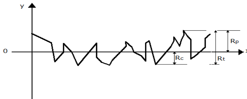
Figure 6.3. Surface rugueuse ( R_t = R_p + R_c )
