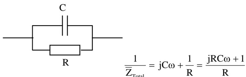
$$\bar{Z}_{\text{total}} = \frac{R}{jRC\omega + 1}$$
