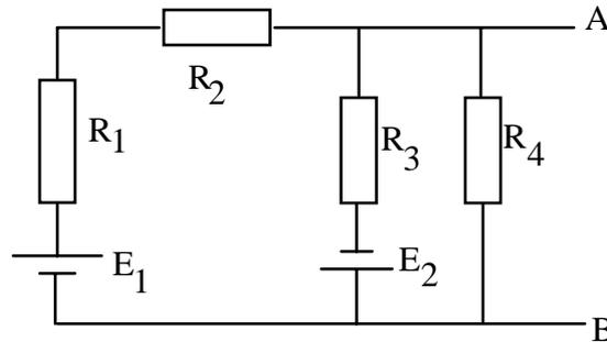
$$R_1 = R_3 = 2\Omega \quad R_2 = 1\Omega \quad R_4 = 3\Omega \quad E_1 = 1V \quad E_2 = 2V$$
