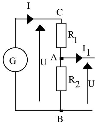
$$U = (R_1 + R_2)I ; I = U / (R_1 + R_2)$$
