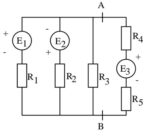
$$\Sigma Y = 1/R_1 + 1/R_2 + 1/R_3 + 1/(R_4 + R_5)$$
