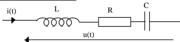
$$\bar{Z} = R + jL\omega + \frac{1}{jC\omega} = R + j\left(L\omega - \frac{1}{C\omega}\right)$$
