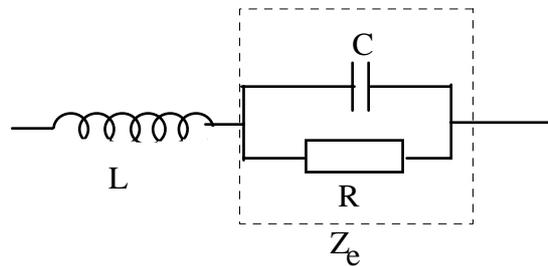
$$\bar{Z}_{\text{total}} = \bar{Z}_e + \bar{Z}_L$$
