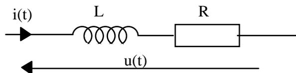
$$\bar{Z} = R + jL\omega \text{ or } \bar{U} = \bar{Z}\bar{I}$$
