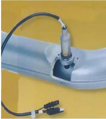
Fig. 4-8 Sonda lambda
