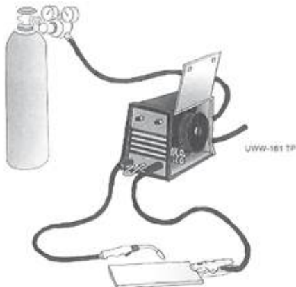
Wire feeder intergrated together with powe source.
