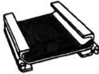
Wear plates and conveyer line pan
