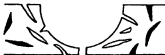
After gouging with Unitor CH-2 382. The oily deposits in the welding area have evaporated.
