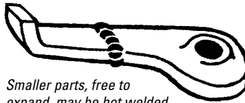
Large complicated parts should be cold welded.
