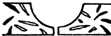
After gouging with Unitor CH-2. The oily deposits in the welding area have evaporated.
