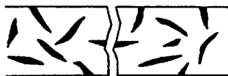
A crack in cast iron. The carbon flakes in the metal are saturated with oil.
