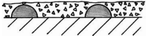
Ceramigrade Abrashield can also be used in combination with the hard surfacing electrode Abratech-330 to fill in between runs. The welding runs give the polymer side support and stability.
