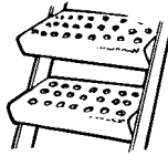
Spot welds on ladder steps
