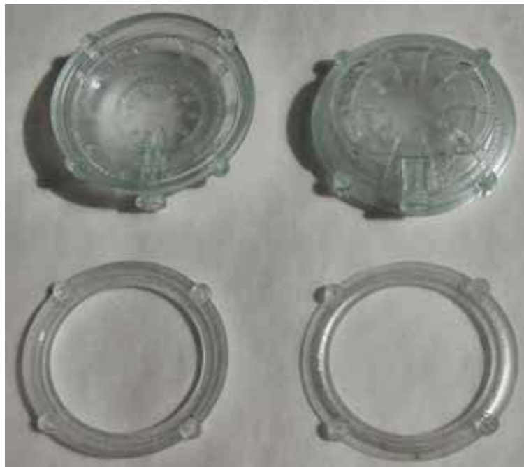
Figure 42 Plastic Parts of Watch 1.0 made by using SLA[71]
