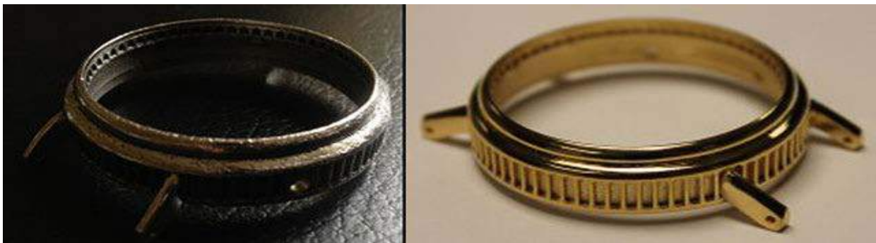
Figure 48: Left: part made with SLM without post processing. Right: same part made with SLM with post processing [89]
