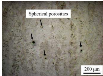
Figure 10 Optical image of spherical porosities (marked by arrows) in an SLM part [52]
