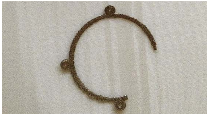
Figure 43 this EBM printing method does not produce the desired parts with the right accuracy [71]
