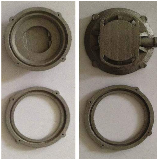
Figure 45 SLM printed part using stainless steel as powder[71]
