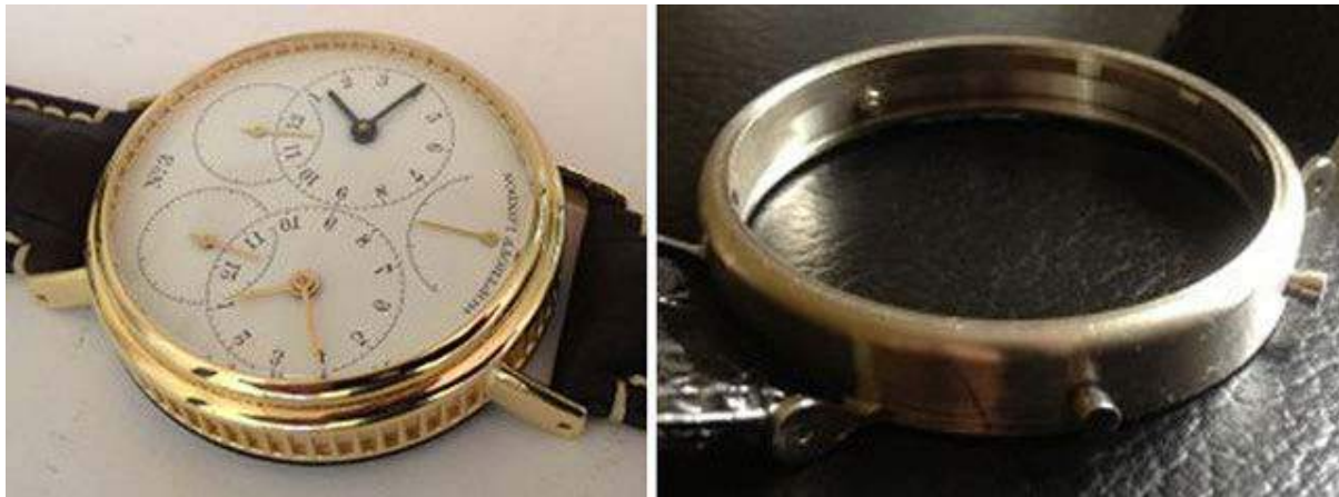
Figure 49: Left: Part Made by SLM. Right: Same Part Made by Traditional [89]
