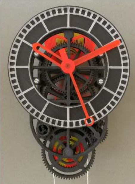
Figure 40: 3D printed mechanical Clock with Anchor Escapement [8]
