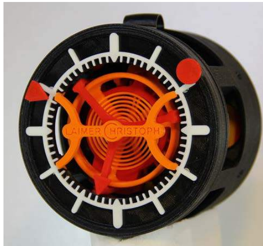
Figure 36: The 3D Printed Tourbillon Watch [8]
