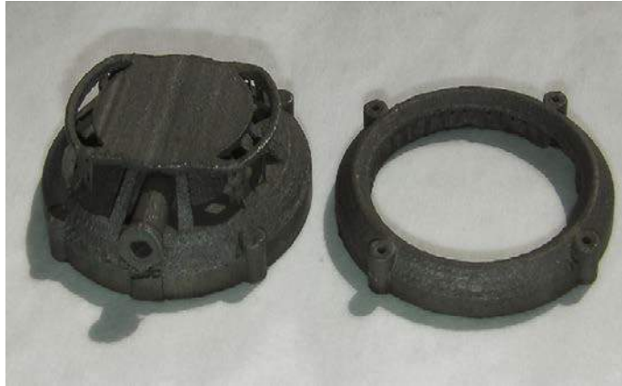
Figure 44 SLM printed part made by using titanium[71]
