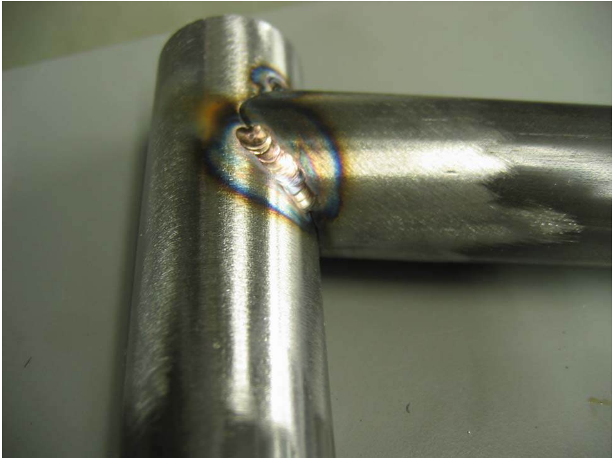
Photo 5: Fillet TIG Weld (4130 Structural Steel Tubing)
