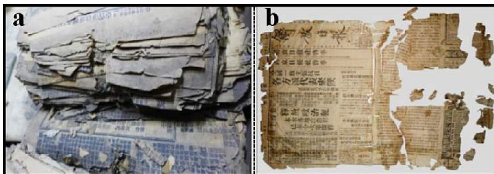
Fig. 1 Typical cases of embrittlement and decay of double-sided printed paper cultural relics: the status quo of newspapers collected in the late Qing Dynasty in the First Historical Archives of China (a); the present situation of newspaper during Xi'an Incident (b)
