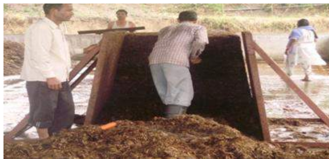
Fig. The set of a Pile former consisting of three steel boards
