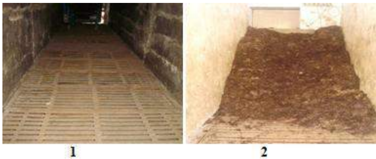
Pasteurization chamber/Tunnel of a Bulk Pasteurization Chamber showing grated panel (1) and compost after phase-I being filled in the chamber for pasteurization process or Phase II (2)
