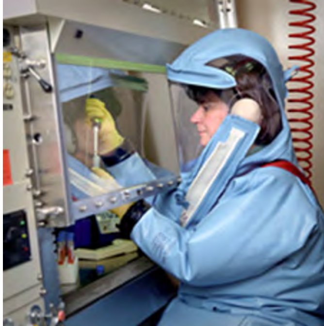
Figure 13.2 A protective suit like this one is an additional precaution for those who work in BSL-4 laboratories. This suit has its own air supply and maintains a positive pressure relative to the outside, so that if a leak occurs, air will flow out of the suit, not into it from the laboratory. (credit: modification of work by Centers for Disease Control and Prevention)
