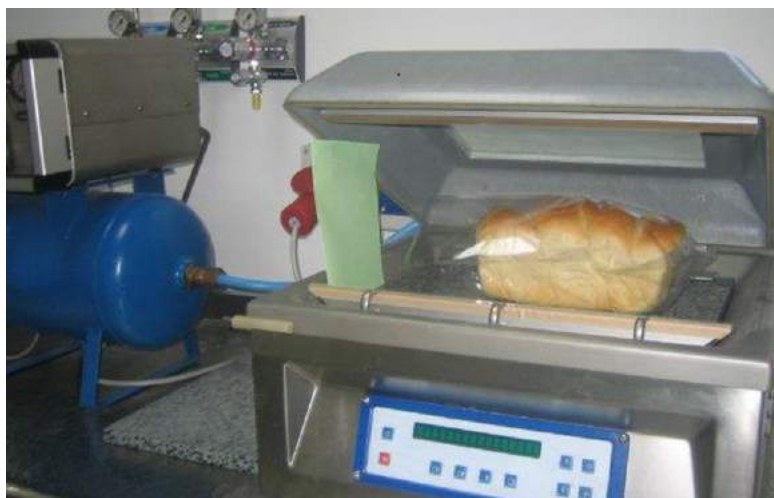
Figure 24. Modified atmosphere packaging MAP (source: IBA Bucharest)
