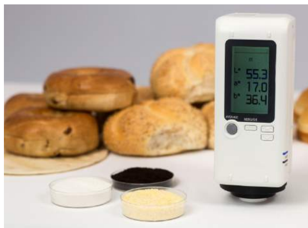
Figure 32. Rapid device for bakery products color determination
