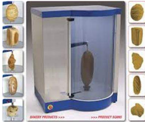
Figure 33. Loaf volume determination (source: www.stablemicrosystems.com )
