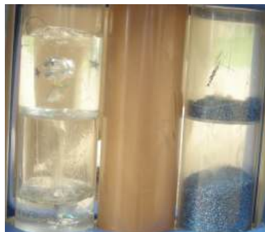
Fig. 16.13 – Picture of Counter-current flow in liquid-gas and solid-gas configurations. The container is made of two compartments. The upper compartment is filled with the heavy phase (liquid, water solution, or small wood particles) by rotating the container. Even though the solid-gas ratio is smaller, it can be noticed that the solid-gas is faster than the liquid-gas flow.
