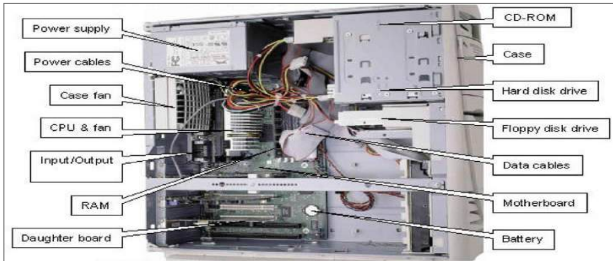
Figure 3.38: Components inside the System Unit
