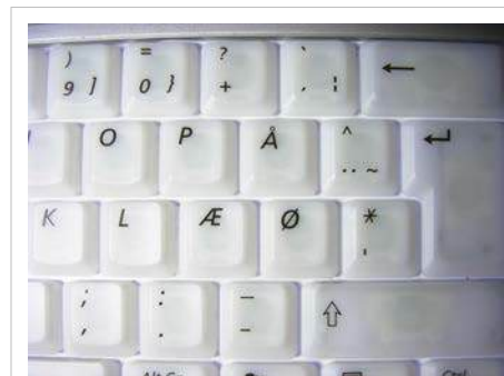
Danish keyboard with keys for Æ , Ø and Å . On Norwegian keyboards the Æ and Ø trade places.
