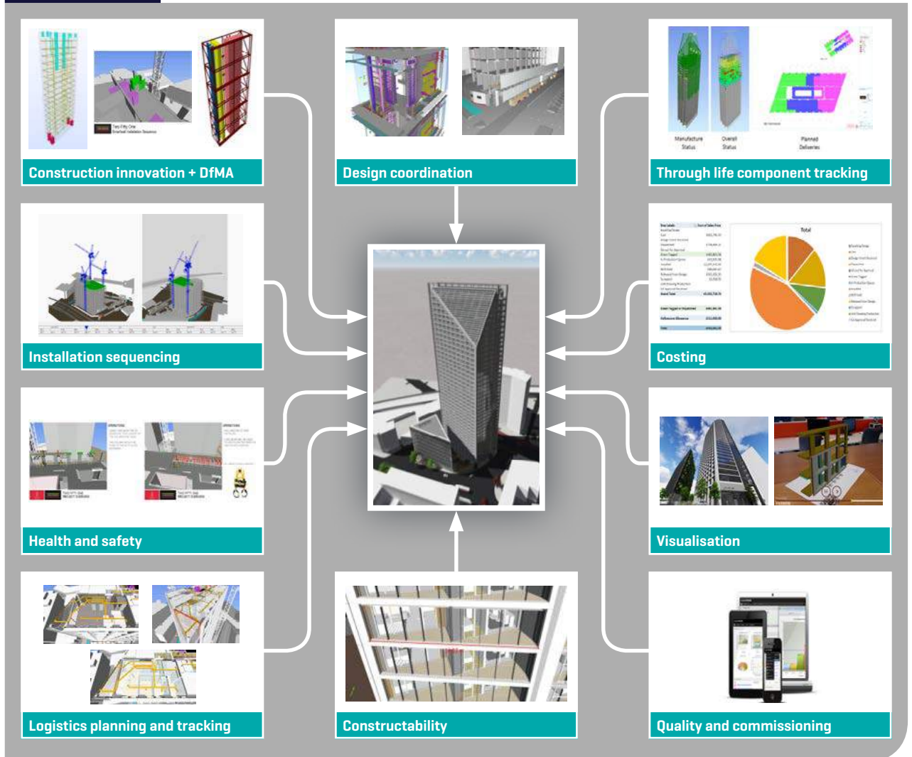
Figure 14 The digital engineering process
