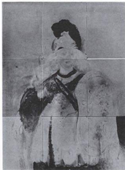
Figure 3. The image of the autoradiograph in Fig. 2 is mainly determined by the radiation from the copper atoms (from the blue-green parts in the painting) and again the mercury of the vermilion.
