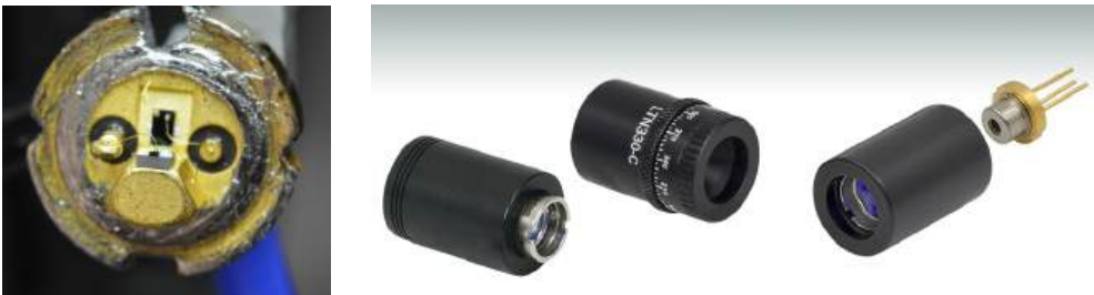
Figure 30.26: (Left) Laser diode with protective housing removed, e.g. using a can opener. (Right) Laser diode collimator.
