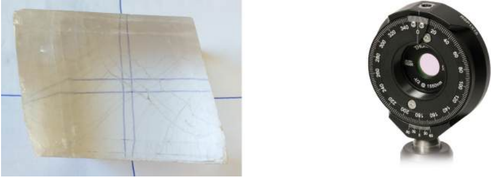
Figure 28.10: (Left) Transmission through a birefringent crystal. (Right) \lambda/2 -waveplate mounted in a rotation stage.
