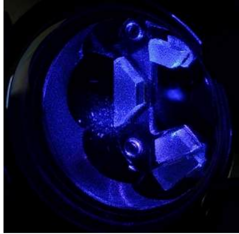
Figure 24.9: Picture of a strontium MOT operated at 461 nm. The atomic cloud, which consists of about 10^6 atoms at 5 mK temperature is visible as a diffuse spot located inside a three-mirror ring cavity.
