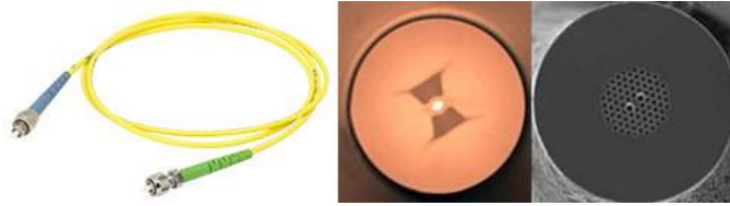
Figure 30.9: (Left) Fiber patch cord, (center) cross section of a bow-tie polarization maintaining fiber, and (right) cross section of a photonic crystal fiber.
