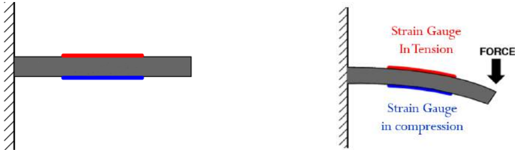
Fig. 2.9(a) Cantilever under no displacement
