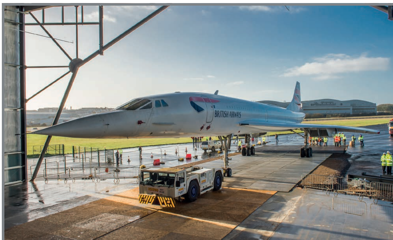
Concorde 'Alpha Foxtrot' being moved into a specially built hangar, at Aerospace Bristol. The hangar was constructed with a movable end wall in order to allow this large aircraft to be placed inside.
