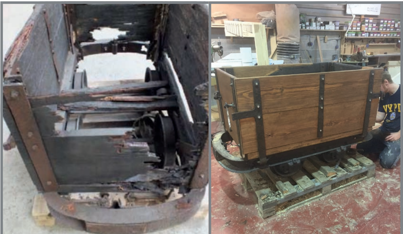
A German-built Orenstein & Koppel (O&K) wagon, found in the vaults beneath Bath Spa Station in 2001. It is believed to be the only known example of its type to have survived. The wagon was restored at BRECO's workshops in Barry between 2015-16 to the specification recommended by conservation consultants, Steph Gillett and George Monger.
