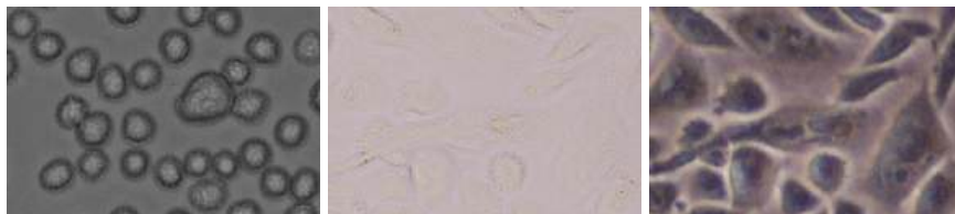
(a) A bright field image dominated by amplitude objects: CHO cells in suspension. (b) A bright field image dominated by phase objects: ultra-thin adherent CHO cells. (c) A phase contrast image dominated by phase objects: age of the same scene shown in 5.9(b). In comparison to 5.9(b), cells are clearly visible, albeit surrounded by halo artifacts.
