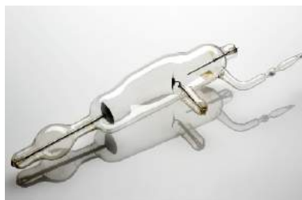
Figure 7.7: Vacuum X-ray tube: The image on the left shows a schematic how electrons are accelerated from the cathode to the anode to generate X-ray photons. The image on the right shows a historic vacuum X-ray tube. Image provided by Science Museum, London, Wellcome Images under Creative Commons by-nc-nd 2.0 UK .
