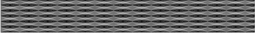
Figure 9.3: Simulated Talbot carpet: interference pattern behind grating G_1 travelling from left to right.
